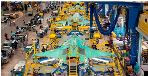
Lockheed Martin's assembly plant in Fort Worth, TX builds F-35 Joint Strike Fighters. (Photo: International Trade Administration)
